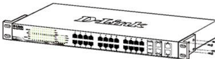
Figure 2.2 – Attach the mounting brackets to the Switch
